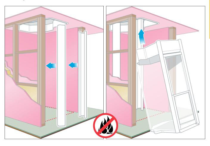
Build door jamb and frame, insulate and cover with fire retardant plasterboard
