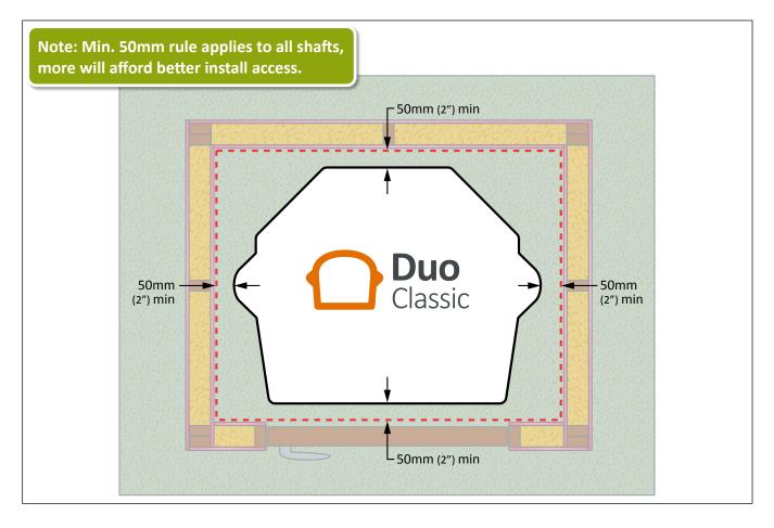
Build 3 walls, insulate and cover with fire retardant plasterboard
